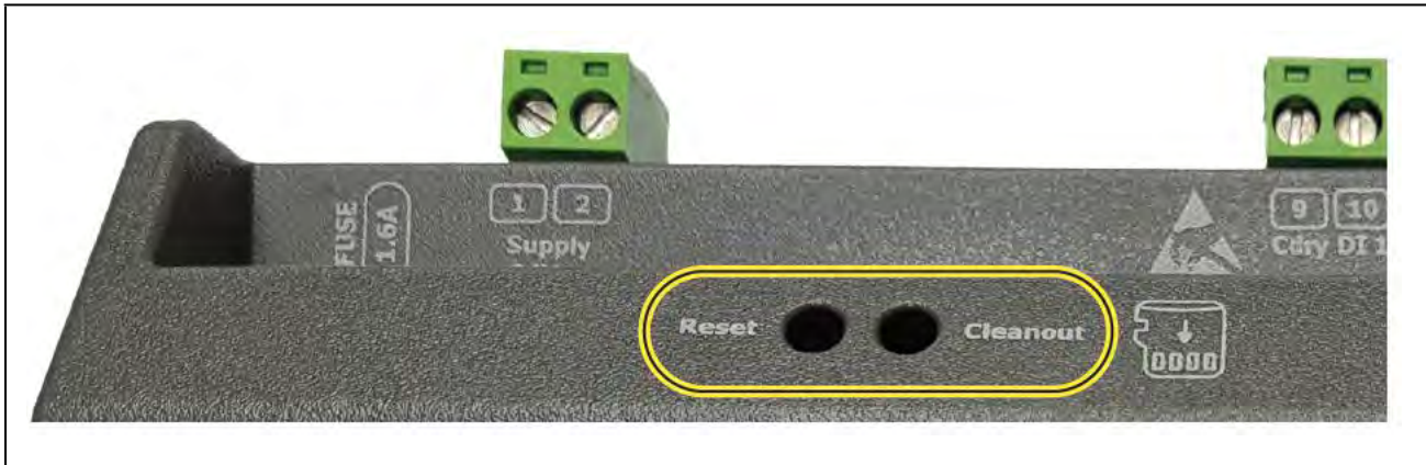
Site Supervisor Reset and Cleanout
