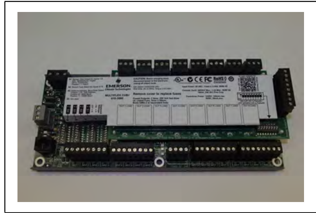
Figure 7-6 - MultiFlex Condensing Unit (CUB)
