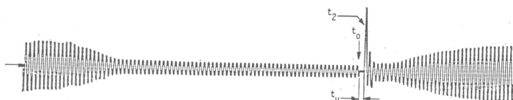
Figure 4a Star-Delta Start - Open Transition
