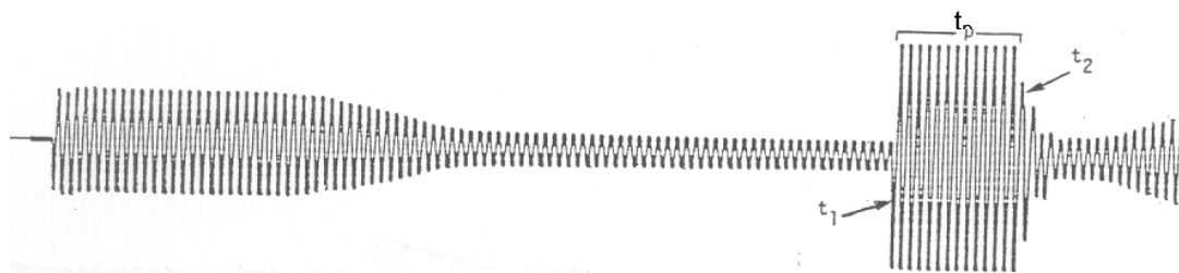
Figure 4b Star-Delta Start - Closed Transition (R7 ≈ 6 Ohms)
