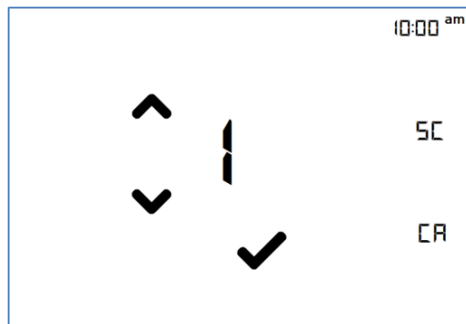
Configuration Menu with Options 0-IDLE, 1-RTU, 2-HP-O, 3-HP-B
