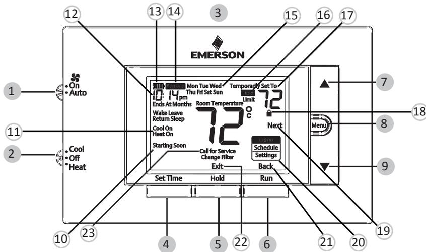
Whenever "Replace" appears in the display, new premium brand AA alkaline batteries should be installed. If the house will be unoccupied for an extended period and either "Replace" or "Replace" is displayed, install new batteries before leaving.
