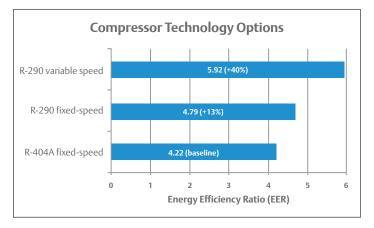
Note: \* Capacity shown at low temperature -10/110 rating point. Variable speed at 3900 RPM for comparison. Compressor capacity range is 1600-5000 RPM.
