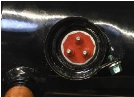
Figure 18: Circle fence with motor terminals
