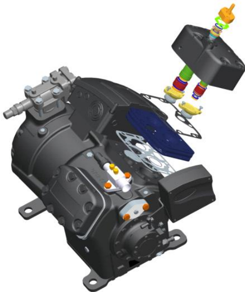
Figure 2: Exploded view of the digital mechanism
