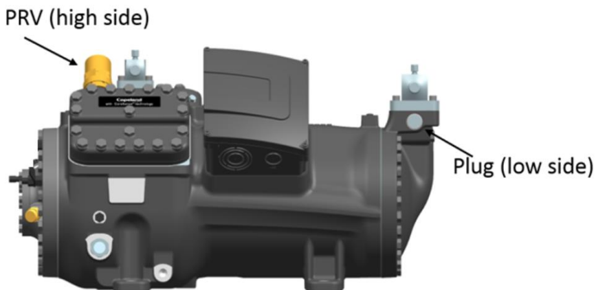
Figure 18: Position of the pressure relief valve – Models 4MTL-35 to 4MTL-50
