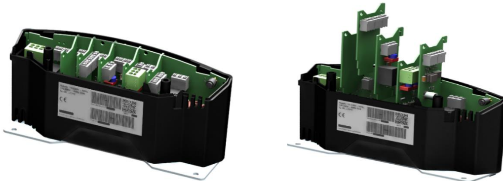
Figure 26: Inside view of the Copeland Compressor Electronics module, with the modular boards
