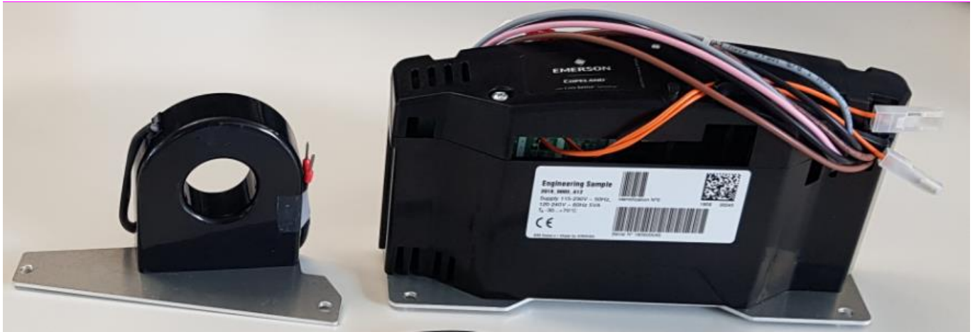
Figure 5: Current sensor and Copeland Compressor Electronics module
