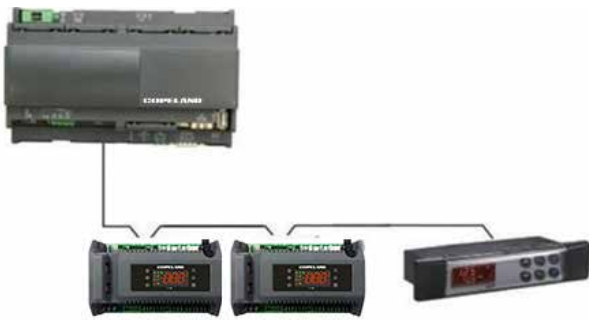
Correct Network Wiring
