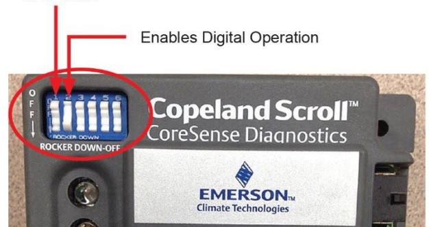
Figure 43 - Medium Temp ZBD*K5E Digital Operation DIP Switch Settings
